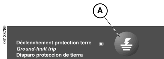
Figure 9: Ground-fault Trip Button
